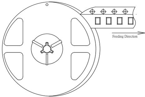
● Dimensions of Reel (Unit: mm)
