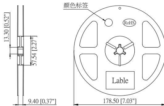
● Dimensions of Tape (Unit: mm)
