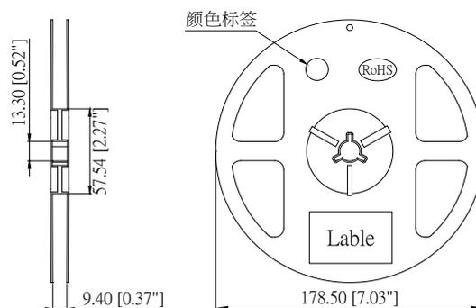
● Dimensions of Tape (Unit: mm)
