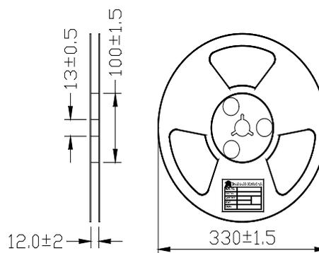
● Dimensions of Tape (Unit: mm)
